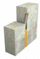
Fire resistant backer rod and standard joint sealant
