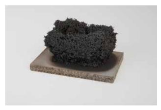
Highly intumescent, fire resistance wrap before (top) and after (bottem) exposure to heat
